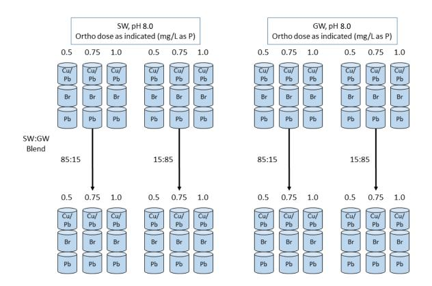
Figure 4. Orthophosphate bench-scale test program
