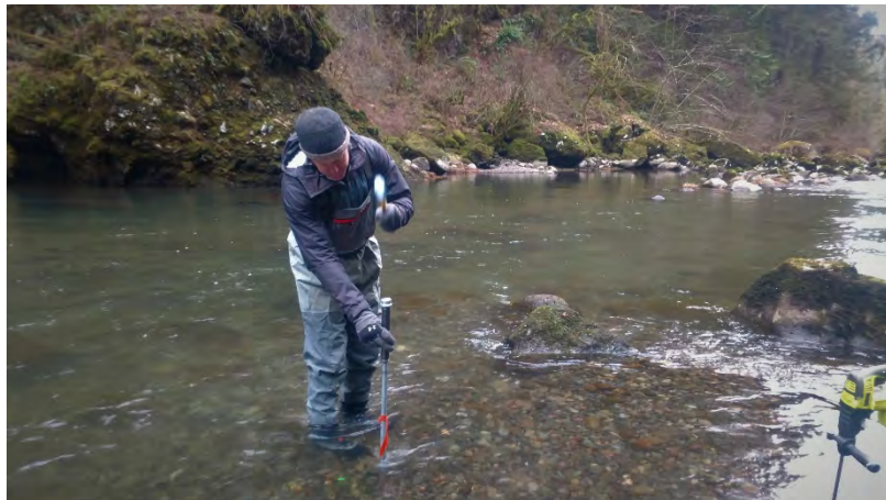
Figure 2. Setting a Scour Monitoring Device. A Rock Drill (lower right corner) is used to Pilot a Path through Gravel to Larger Substrate or Bedrock
