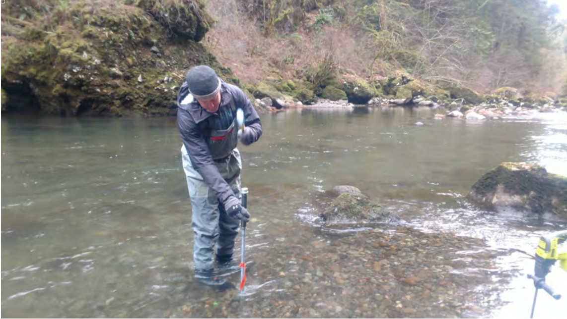
Figure 13. PWB Staff Installing a Gravel Scour Monitoring Device in the Lower Bull Run River Adjacent to a Chinook Salmon Redd
