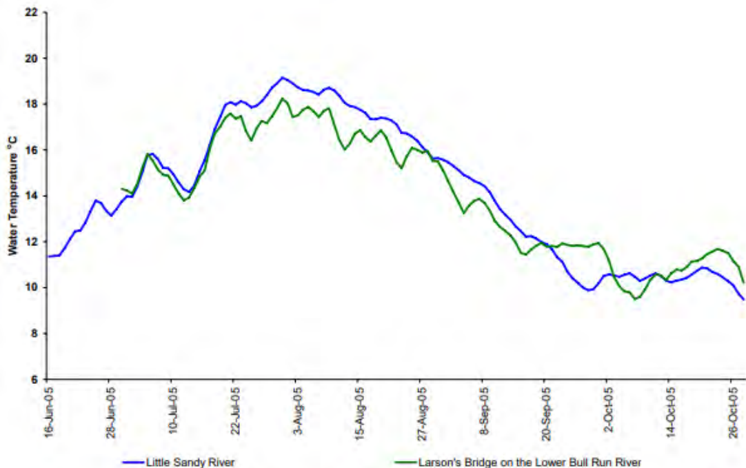
[from 2008 Bull Run Water Supply Habitat Conservation Plan] Figure 8-4. Comparison of Actual 7-Day Maximum Water Temperatures for the Little Sandy Rivers with Predicted 7-Day Maximum Average Temperatures for the Lower Bull Run River, June 16–October 24, 2005.
