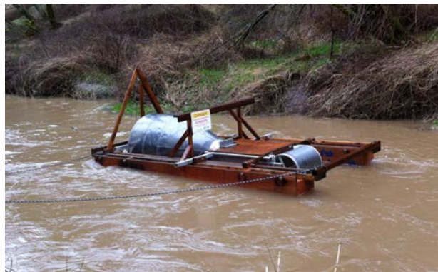
Figure 3. A trap made largely of wood was used in Beaver Creek to discourage metal theft.
