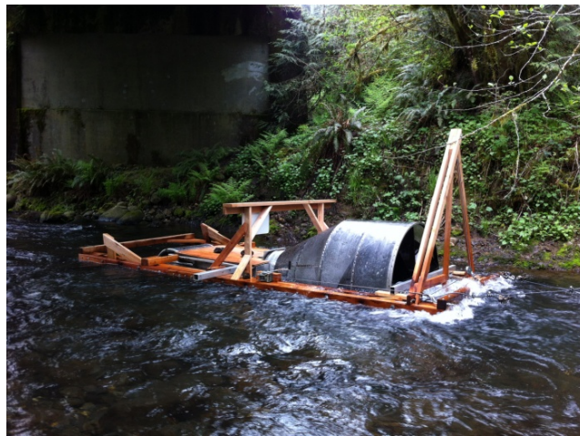
Figure 3. After trap parts were stolen, Gordon Creek was monitored by mounting a rotary screw and livewell to a wooden frame standing on the streambed.
