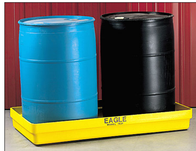
(h) INADEQUATE Secondary Containment Skid for 55-Gallon Drums (Only has 32 gallons of Containment Capacity – 60 gallons Required)
