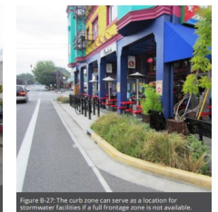
Figure B-27: The curb zone can serve as a location for stormwater facilities if a full furnishing zone is not available.
