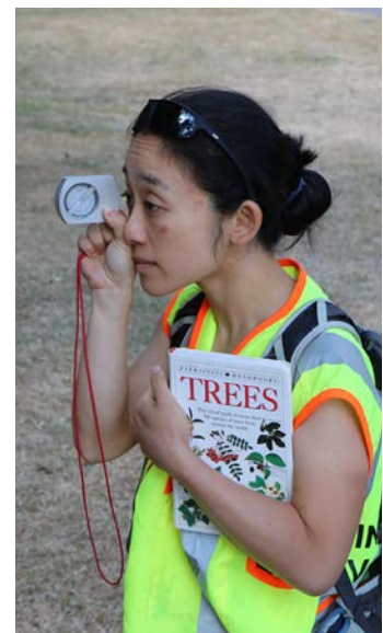
Keep both eyes open when using the clinometer; to see both the instrument scale and the tree.
