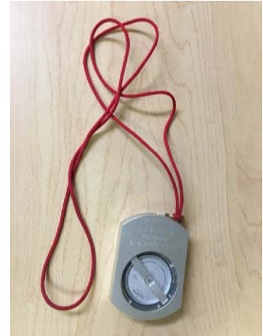
A clinometer is used for measuring tree height
