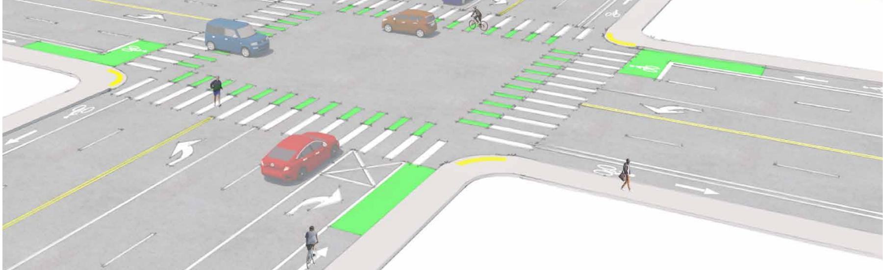
This concept separates bicyclists/pedestrians on SE 122nd from right-turning drivers, maintains bike lanes along the curb to the intersection, and has minimal impacts to the existing curbs/utilities. The reduced cost of this option would provide additional funding for improvements elsewhere along the corridor.
