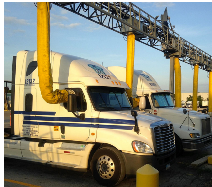
Picture 6.2: "HVAC Hookup" Two white freight tractors connected to an external HVAC system. The HVAC system is yellow and enters through the windows of the freight vehicles. [source: unknown]
