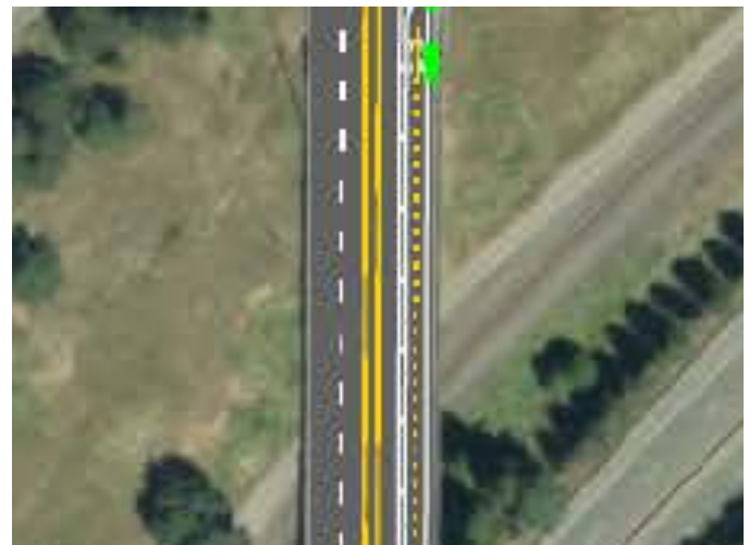
Design of the two-way protected bicycle lane on the bridge over the railroad and I-84.
