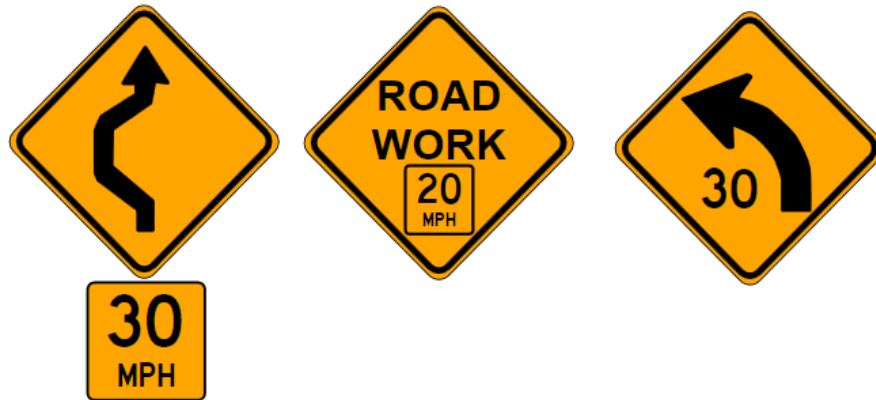
Figure 6.6 Warning Signs with Advisory Speeds
