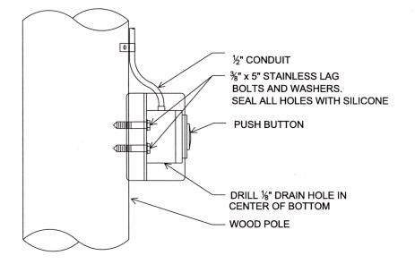
$\underline{\text{NOTE}} = \text{FOR WOOD POLE INSTALLATION,REMOVE RIVETS \&}$  INSTALL BOX WITH  $\frac{1}{2}$ " HUB FACING UP.
