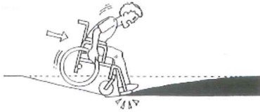
Figure 7-23. Overlaying existing asphalt without milling away the old asphalt can create steep slopes on either side of the centerline.
