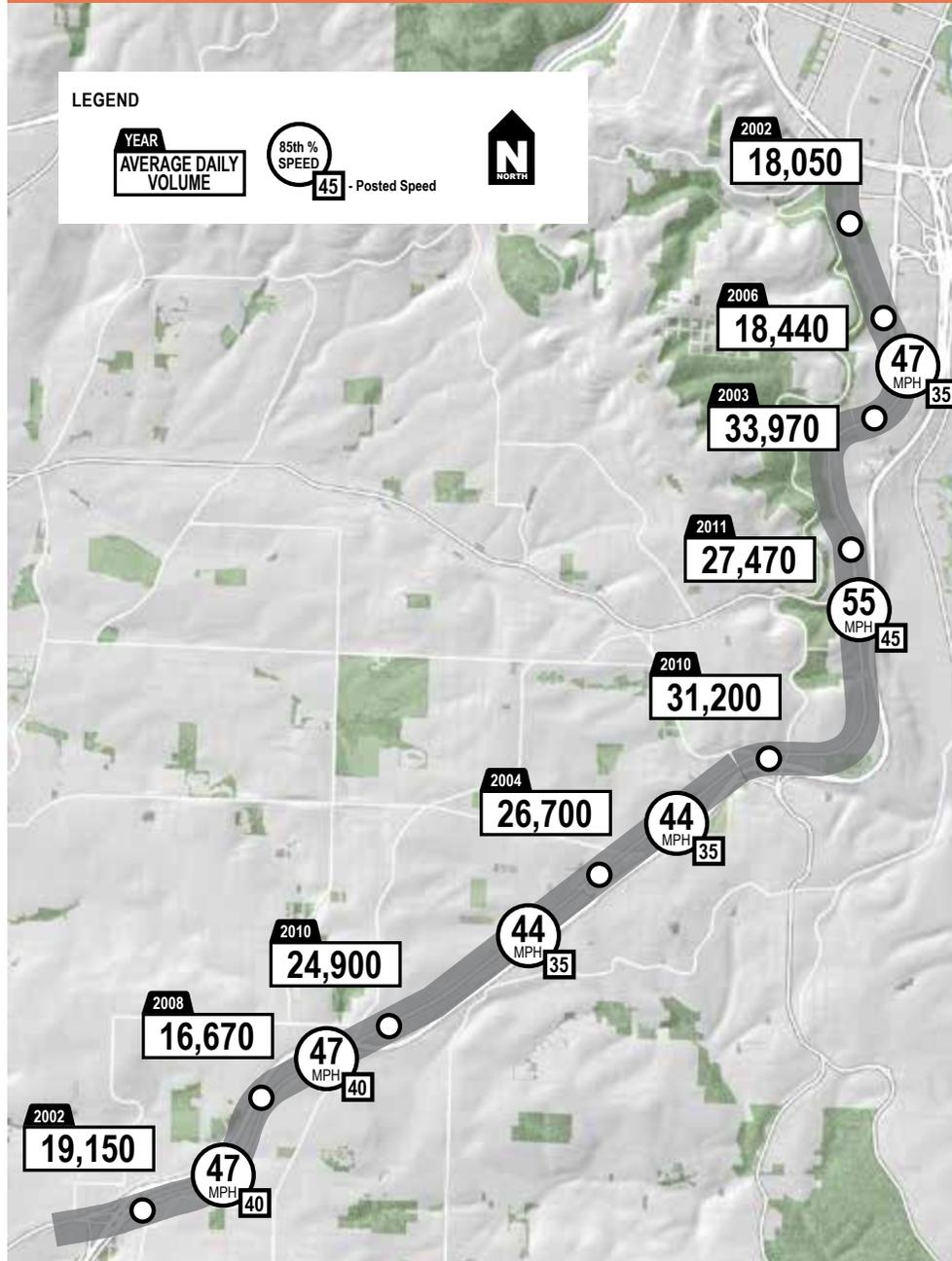
This map provides information about the relative quantity of vehicles moving on different parts of Barbur, as well as an indication of the 85th percentile speed.
