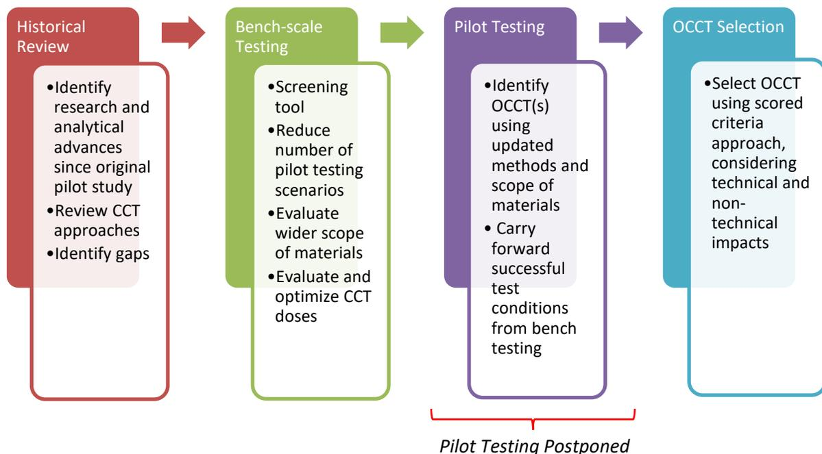
**Figure 1. Lead Corrosion Control Strategy Decision Tree**
