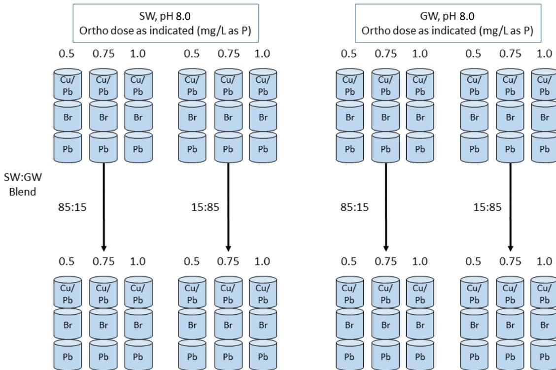
**Figure 4. Orthophosphate bench-scale test program**
