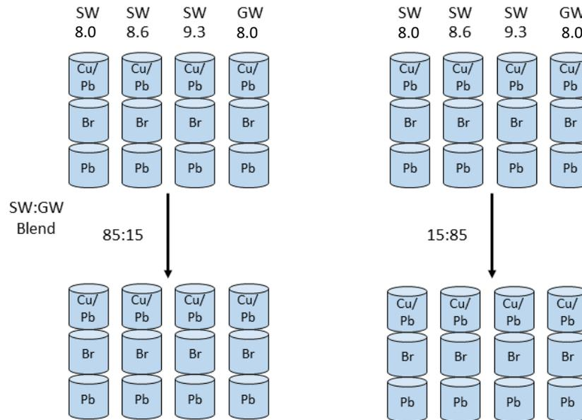
**Figure 3. pH/alk bench-scale test program**
