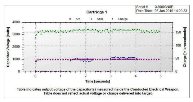
IMAGE ATTACHMENT (2994223) TASER PULSE GRAPH ARC
