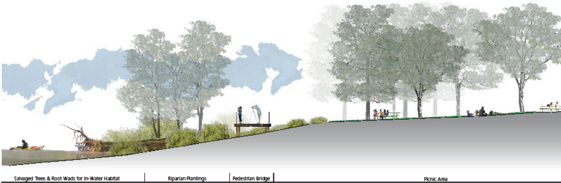
Cross-section 'C' at off-channel habitat improvements and pedestrian bridge connecting into the cottonwood draw
