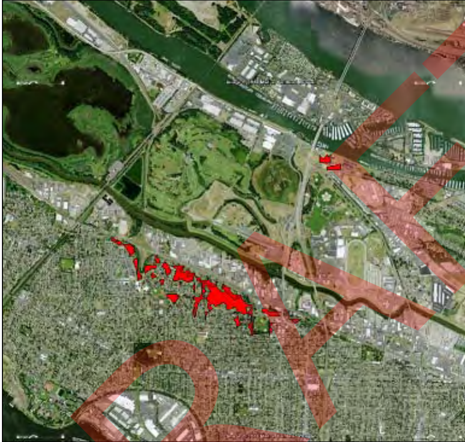
Figure 4. PIR Full Track Race Daytime Broadband Residential Code Exceedance Areas for 103-dBA Trackside Event (10 vehicles), No Meteorology
