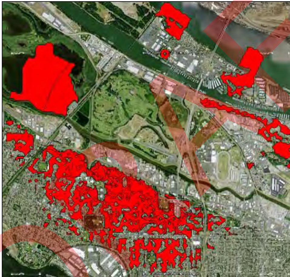
Figure 5. PIR Full Track Race Daytime Broadband Residential Code Exceedance Areas for 113-dBA Trackside Event (10 vehicles), No Meteorology
