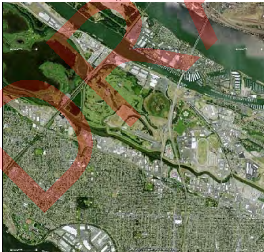
Figure 2. PIR Late Night Drag Nighttime Broadband Residential Code Exceedance Areas for 90-dBA Trackside Event, No Meteorology
