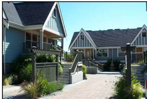
Multidwelling projects (with, respectively, 10.5' and 12'-wide driveways) in Seattle, which allows multidwelling driveways to be as narrow as 10'. This allows for less impervious surface and more pedestrian-friendly street frontages.
