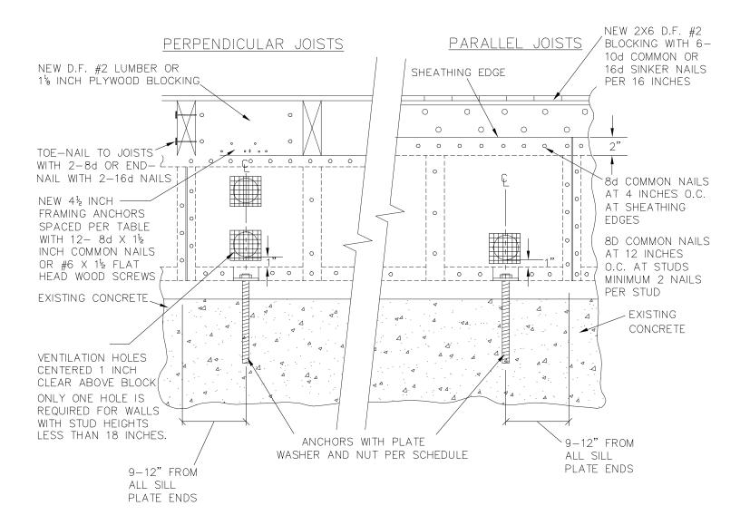
(9) cripple wall bracing- interior elevation
